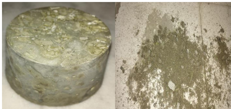
Fig 3: Casting and Failure of Cement Palm Block
